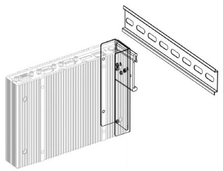
7. If necessary, establish protective grounding for the mounting package. The KeContact M20 is installed on the top hat rail.
