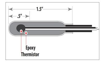
Note, the most active portion of the sensor is the first 1/2" of the 1-1/2" long stainless steel probe.
