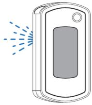
7. Once the location is validated, apply Velcro or an adhesive strip, and place sensor.
