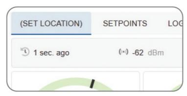
6. If the timer reads 1 second or less, the location is ideal. Below 10 seconds is good. If 20 seconds or more, consider moving or changing the orientation of the sensor.
