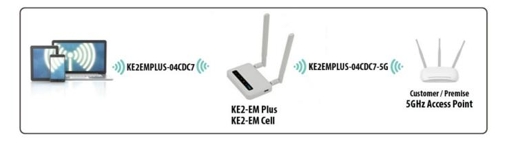
• User connects their smart device to the KE2EMPLUS-04CDC7 2.4GHz Wi-Fi network to access the KE2-EM Plus. The 5GHz radio is used to create the Wireless Bridge to the existing Wi-Fi network.
