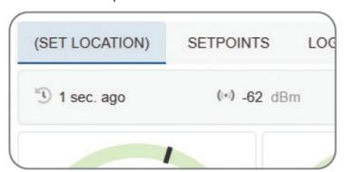
4. The timer in the top left shows how often the wireless sensor is checking in with the KE2-EM. This helps determine optimal sensor location.
