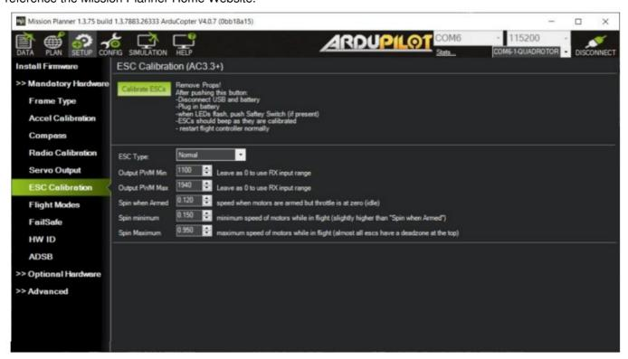
**Note:** program the "ESC Type" to "Normal" for synchronization of autopilot gyros and ESC control frequencies (400 Hz dynamic).
