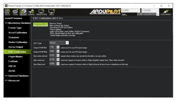
Note: program the "ESC Type" to "Normal" for synchronization of autopilot gyros and ESC control frequencies
