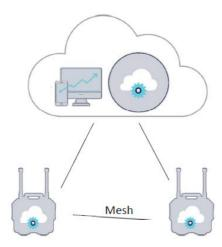
Additionally, the Base Station implements a 2.4GHz wireless mesh communication network between itself and its peers. This mesh provides the ability to communicate locally between Base Stations. This mesh creates multiple paths to the cloud such that not all Base Stations are required to be connected directly to the internet, but instead can forward their outbound traffic to a peer. The mesh also allows for running edge analytics algorithms.
