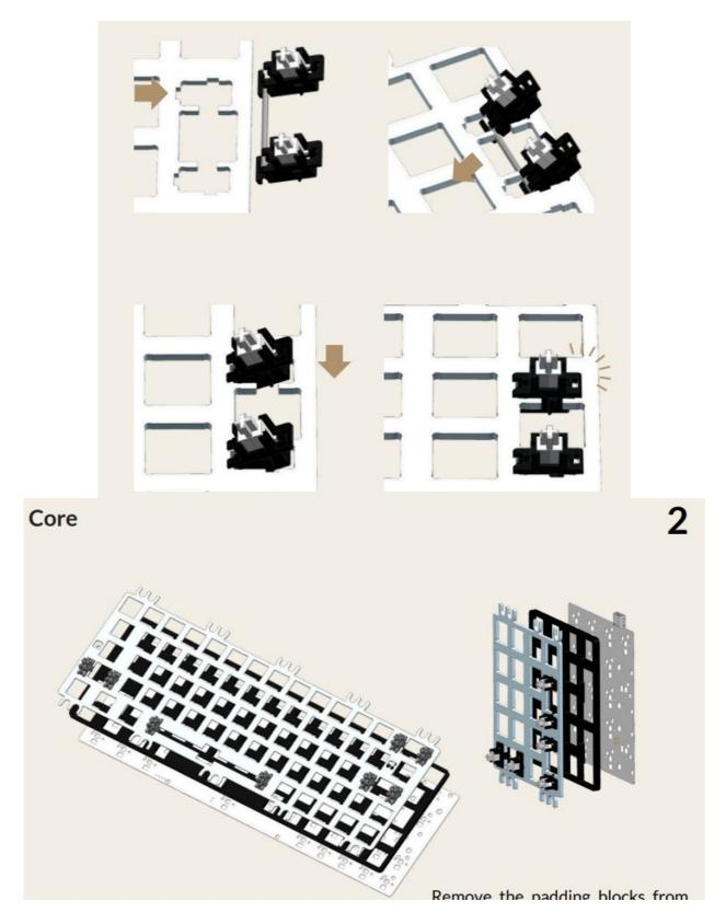
Remove the padding blocks from the Poron foam, and then assemble the both cores by aligning the plate, foam, and PCB.
