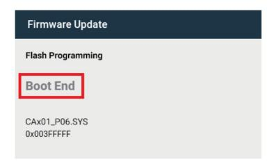
After approximately 1 minute a "Boot End" message will be shown in the LCD display, indicating that the first stage of the update has been successful.
