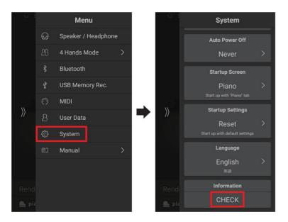
If the Firmware version number is greater than or equal to the update zip file filename, no further action is necessary.
