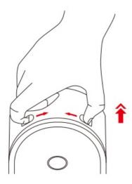
2. Remove all fittings by lifting the drum upwards.
