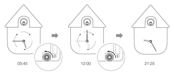
4. Close the battery cover after the time is set correctly. Do not press "SET" button during the process. **Otherwise**, please take out the batteries and reset the time by following steps (1)- (4) above.
