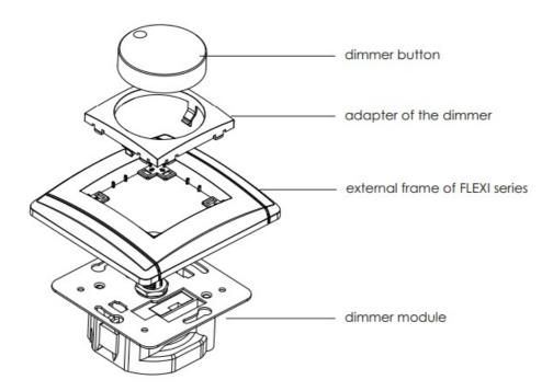
Installation instructions for electronic light controller mechanism in multiple frames
