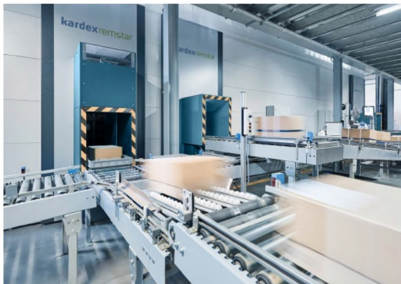
Order consolidation with automatic conveyor connection
