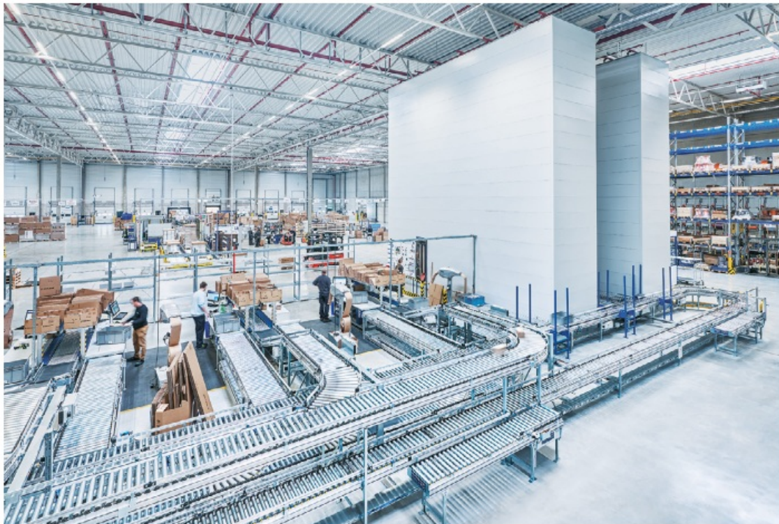
Vertical Buffer Module Kardex Compact Buffer with automated conveyor connection
