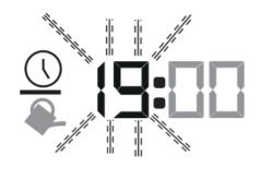
As soon as the battery is inserted, the display, after a short self-tes t, changes directly into the settings mode for the current time. The hours of the time display are flashing.
