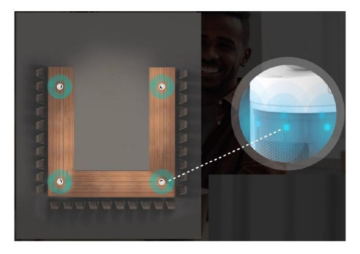
• The 4×8 microphone array combination, achieves a wider range of better sound quality, with built-in beamforming, echo cancellation, voice noise reduction, and howling suppression.
