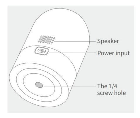
The 1/4 screw hole at the bottom is designed to ensure the device is widely compatible with photography accessories and provides stable installation.
