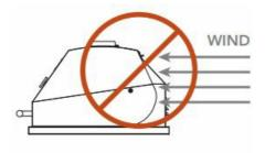
Do not place the grill in a location where the rear hood openings are likely to be exposed to strong wind. A wind break wall is recommended for installations where the prevailing wind may be a problem.
