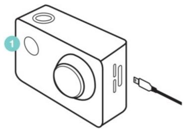
2. Connect the Micro HDMI end to the port on the camera and HDMI end to HDMI port on the TV.
