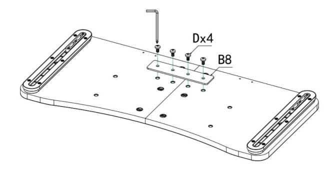
Place part B8 over the screws C on part B1 and fasten with 4 screws D.
