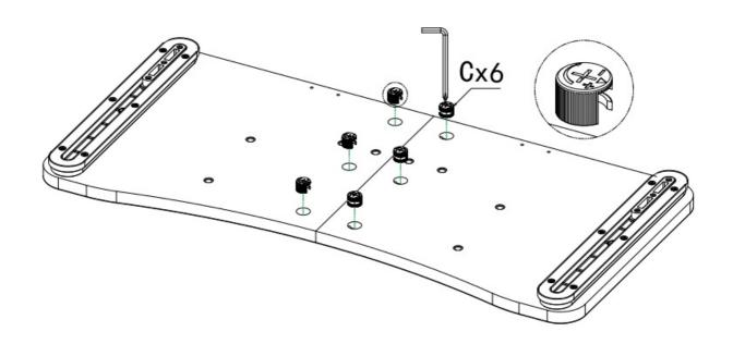
Insert 6 screws C through the top of part B1.
