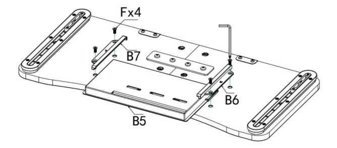
Attach part B7 to the assembly using 4 screws F, with part B5 underneath and part B6 on top.
