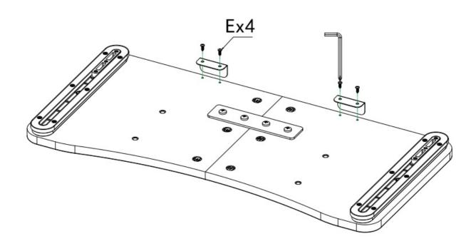
Secure part B8 to part B1 using 4 screws E.
