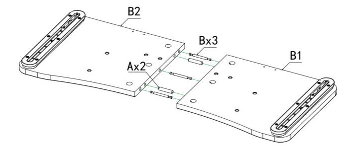
Align parts B2 and B1 and secure them using 2 screws A.
