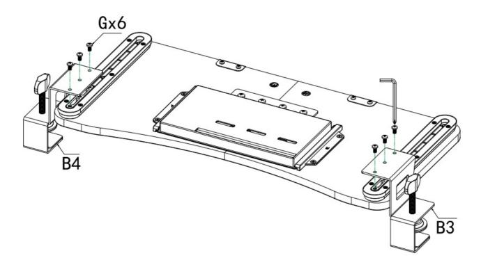
Attach part B4 to the side of the assembly using 6 screws G, then attach part B3 to the opposite side.
