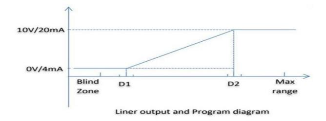
The analog output can be set through RS485 interface, the setting procedure is as follows,
