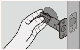
Hold the latch in front o the bore hole, with the latch face flush against the door edge. Is the siotted hole contered in the door hole?
