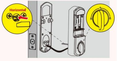
D Attach interior assembly to mounting plate and tighten 3 screws.
