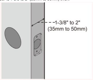
D Make sure the hole in the door frame is drilled a minimum of 1" (25mm) deep, to leave enough space for the "deadbolt to extend into the door frame when the door is locked.
