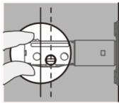
Rotate and pull the latch as shown to extend latch.
