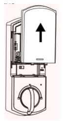
B Insert the cable into the connector. Push the connector in firmly until it is completely attached.
