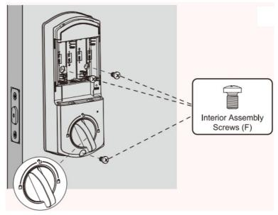
E Insert the Z-Wave module and make sure the network Module is securely plugged in. **Note:** Before inserting the module, make sure the lock does not have a battery installed.
