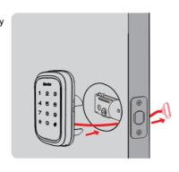
C Secure the mounting plate with the supplied screws. Do not overtighten screws.
