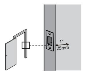
**Notes:** Make sure the door frame is aligned with the door and there are no obstructions stuck in the door frame.
