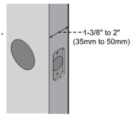
• D Make sure the hole in the door frame is drilled a minimum of 1" (25mm) deep, to leave enough space for the deadbolt to extend into the door frame when the door is locked
