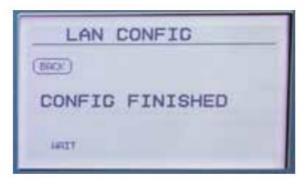
Power cycle the controller by disconnecting the main power again. Wait 20 seconds then reconnect the power. Turn the dial to **CONNECTIVITY.**
