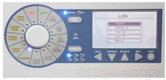
Wait about 30 seconds for the Site Master to be connected online. Once connected, the LCD screen will display STATUS KRAIN SERVER. The controller is successfully connected.
