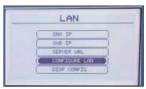
**3d** Press the INCREASE button to change **NO** to **YES**. Press **OK**. Wait several seconds until you see **CONFIRM CONFIG NO**.
