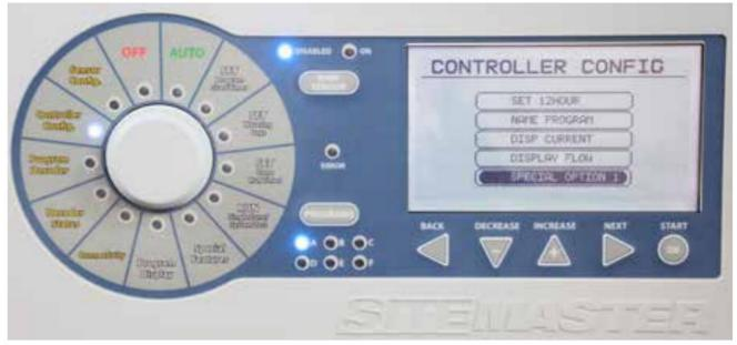
2. Use the NEXT button to find the line GSM LAN 30. Use the INCREASE button to change the value to 002. Then use the NEXT button to go to GSM LAN CONFIG 31. Change the value to 001.
