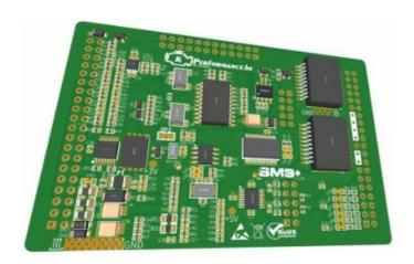
The SM3+ Module R1.5 is a circuit based on MegaSquirt 3 and pinout of the KdFi1.4 modules. It is designed to be backward compatible with MS2 KdFi1.4 users and boards. The module is 100% AEC-Q100 compliant and includes a performance Wideband Lambda Controller with a Bosch LSU 4.9 sensor.
