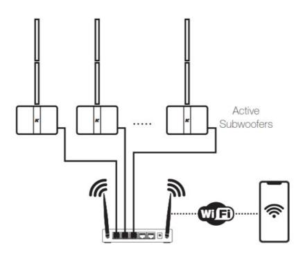
The simplest local network of Thunder-KS active subwoofers requires the implementation of an Ethernet switch. When an access point is available, the network of Thunder-KS active subwoofers can be easily managed with the K-array Connect mobile app over the LAN.
