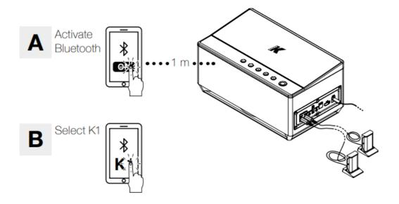
When turned on, the K1 will automatically connect to the last connected device if available; if not, the K1 will enter pairing mode.
