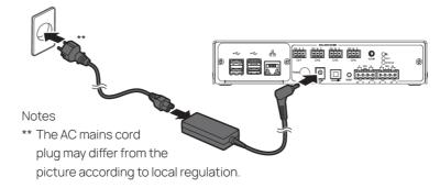
Once properly plugged, switch on the amplifier pushing on the power button: when the unit is operating the front and back LEDs light on green.
