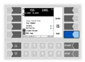
2. The **Tour Menu** screen will appear. Select **Emptying System** with the selection keys and press ENTER. The pump will suck air to press the remaining milk from the system into the trailer.
