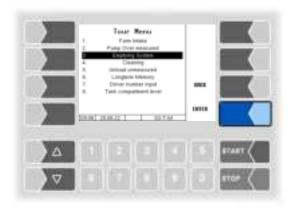
3. Wait until the pipe icon will be displayed as empty. The system will automatically stop after the configured duration is over. You can stop the process at any time by pressing FINISH. If the system stops automatically without clearing the system completely, restart the process.
