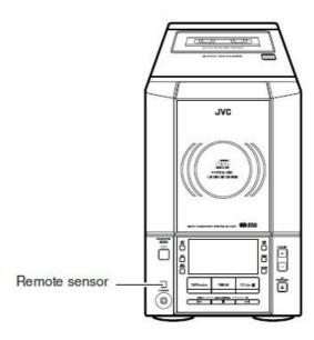
• The Remote Control makes it easy to use many of the functions of the System from a distance of up to 7 m away.
