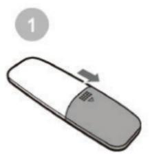
2. Load one AAA 1,5V battery (not included) into the battery compartment, observing the polarities inside the battery compartment.
