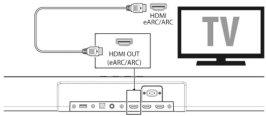
Connect the HDMI cable from unit's HDMI OUT (TV eARC/ARC) socket to the HDMI (ARC) socket on your ARC compliant TV.
