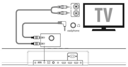
Use a 3,5mm to 3,5mm audio cable to connect the TV's or external audio device headphone socket to the AUX socket on the Soundbar.
