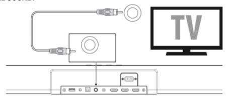
You also can use the COAXIAL cable to connect the TV's COAXIAL OUT socket and COAXIAL socket on the Soundbar.
