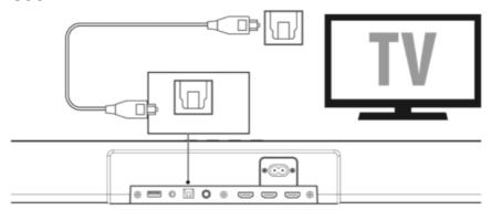
Connect an OPTICAL cable to the TV's OPTICAL OUT socket and the OPTICAL socket on the Soundbar. **USE THE COAXIAL SOCKET**
