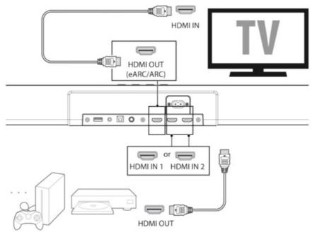
Use an **HDMI** cable to connect the soundbar's HDMI OUT (TV eARC/ARC) socket to the TV's HDMI IN socket. Use an **HDMI** cable to connect the soundbar's HDMI IN (1 or 2) socket to your external devices (e.g. games consoles, DVD players and Blu-ray).
