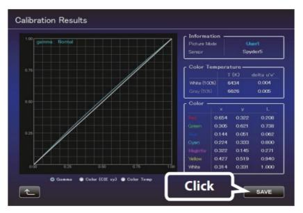
The calibration result includes the characteristics of the screen. It is recommended to set the Screen Adjust function of the projector to off after calibration.
