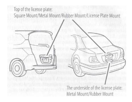
When you decide on the camera installation position, clean the surface of the installation position. Using a commercially available cleaner, wipe the dirt, moisture, and oil away from the surface on which the camera bracket is to be attached
