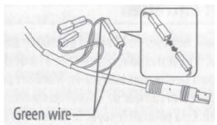
• After disconnecting the terminal, wrap the terminal with an insulating tape as illustrated below.
