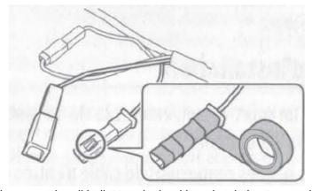
• To prevent a rattling noise, wrap the all bullet terminals with an insulating tape as illustrated below.
