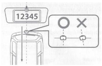
Install the camera at the center of the vehicle and not to hide the license plate. And also install straight toward the forward/reverse direction of the vehicle. Be careful not to lean the camera toward other directions of the vehicle, etc.
