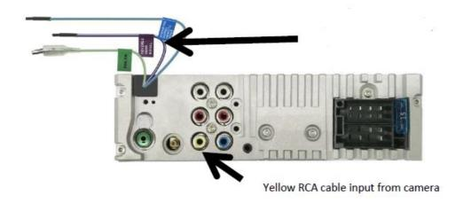
Reverse input from Piggy-Back loom/ Reverse lamp connects into Purple/White wire marked 'Reverse'. Yellow RCA cable input from camera If the image on your head unit screen is reversed, flip the image in your head unit menu settings. If your head unit doesn't have an image flip function, cut the small green/blue wire loop on the camera harness to reverse the image.
