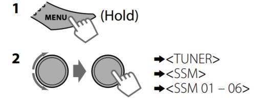
"SSM" flashes. When all the stations are stored, "SSM" stops flashing. To preset <SSM 07 - 12>/<SSM 13 - 18>, repeat steps 1 and 2.
