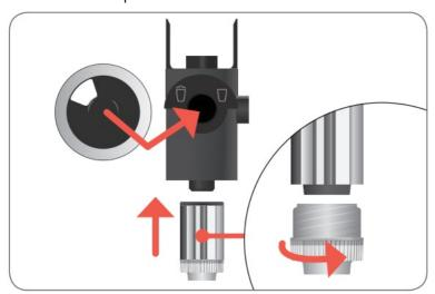
I Ensure that all individual parts are correctly and firmly connected to ensure optimum operation of the professional fine foam frother.
