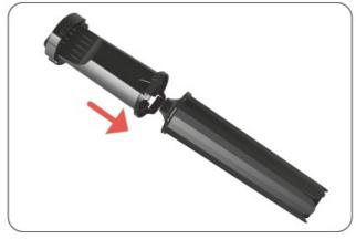
Insert the filter cartridge with its extension into the water tank.
