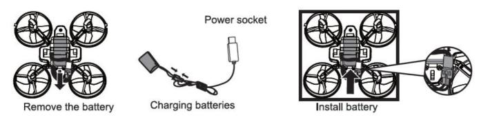
Take out the aircraft battery, then connect the charging head of the USB charging cable to the battery charging socket, and connect the USB terminal to the power supply for charging.
