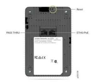
You can plug the Eth0+PoE port into the PoE switch or PoE brick to power on the AP12. The port uses a DHCP IP address for management. Pass-through ports marked Pass Thru act as a patch from the back to the side port. You can use a pass-through port in cases where you need to connect a device behind a wall mount, such as a TV in a hotel.
