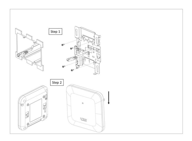
Step 1Mount APBR-U to the box using two screws and the #2 holes. Make sure Ethernet cable extends thru the bracket.Step 2Slide the AP with shoulder screws on the APBR-U until the lock is engaged
