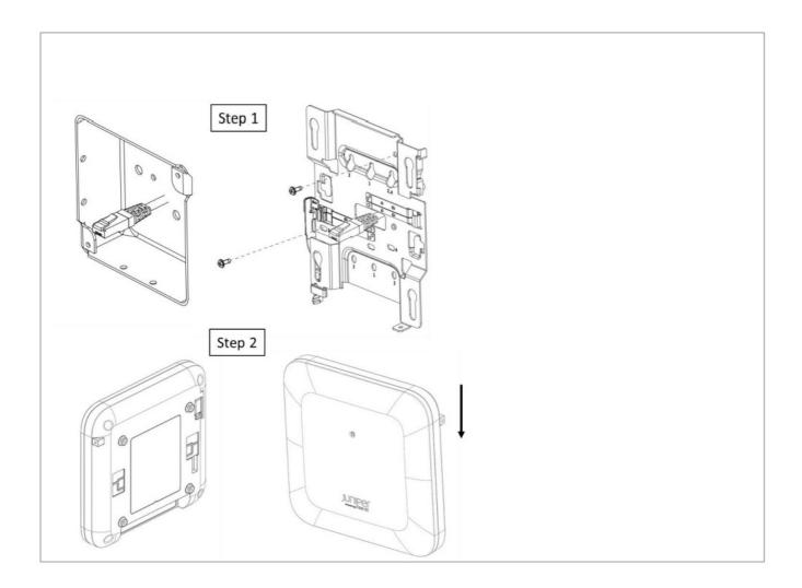
**Step 1** Mount APBR-U to the box using two screws and the #3 holes. Make sure Ethernet cable extends thru the bracket.
