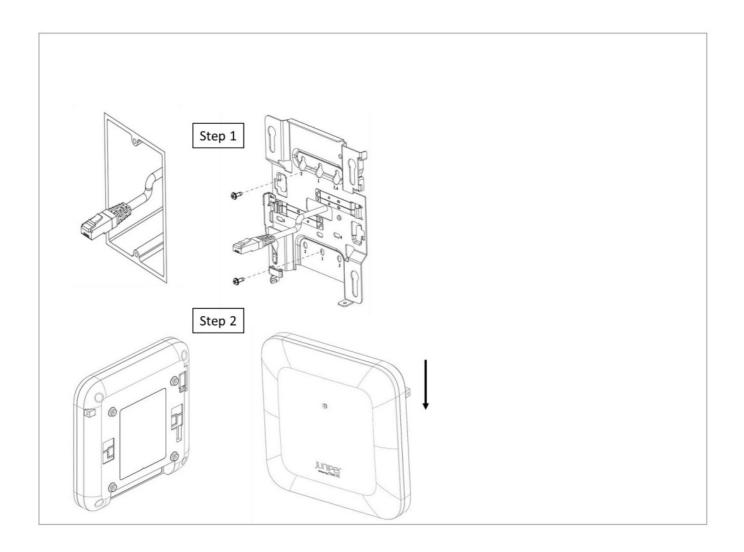
**Step 1** Mount APBR-U to the box using two screws and the #1 holes. Make sure Ethernet cable extends thru the bracket .
