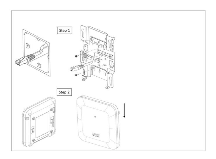
Step 1Mount APBR-U to the box using two screws and the #4 holes. Make sure Ethernet cable extends thru the bracket.Step 2Slide the AP with shoulder screws on the APBR-U until the lock is engaged
