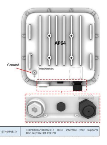
Ground should be connected to Earth ground using wire that is 8AWG or larger diameter.
