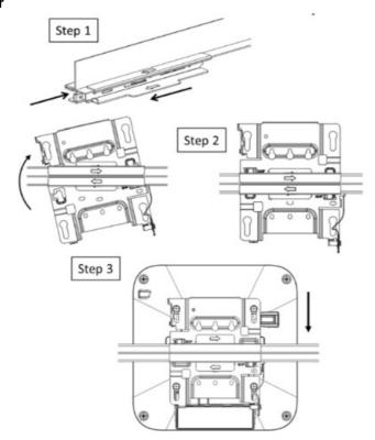
Step 1 Mount the APBR-ADP-RT15 to the t-bar
