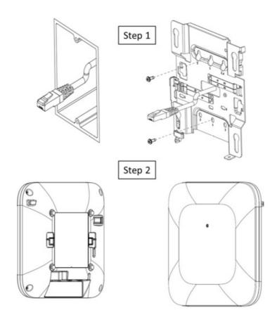
**Step 1** Mount APBR-U to the box using two screws and the #1 holes. Make sure Ethernet cable extends thru the bracket.
