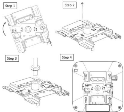
Step 3. Install the APBR-ADP-T12 to the APBR-U. Rotate to lock.
