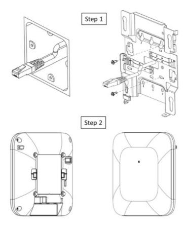
**Step 1** Mount APBR-U to the box using two screws and the #4 holes. Make sure Ethernet cable extends thru the bracket.
