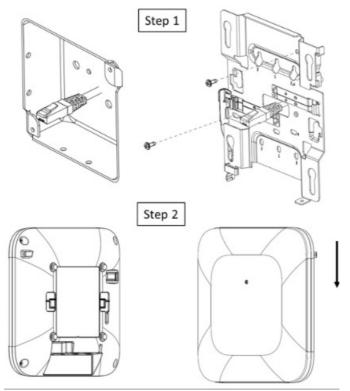
**Step 1** Mount APBR-U to the box using two screws and the #3 holes. Make sure Ethernet cable extends thru the bracket.
