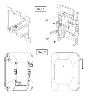
**Step 1** Mount APBR-U to the box using two screws and the #2 holes. Make sure Ethernet cable extends thru the bracket.
