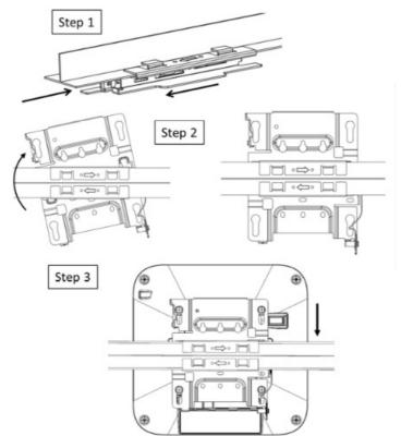
Step 1 Mount the APBR-ADP-WS15 to the t-bar
