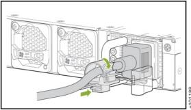
**WARNING:** Ensure that the power cord does not block access to router components or drape where people can trip on it.
