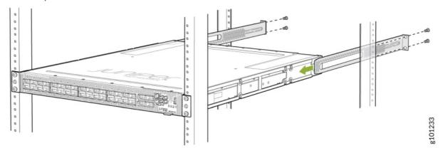
9. Verify that the mounting brackets on each side of the rack are level.
