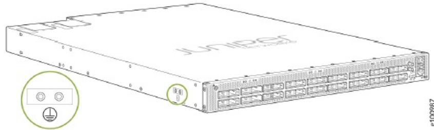
Figure 8: PTX10001-36MR Grounding Points
