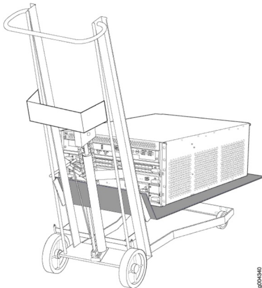
Figure 6: Load the MX240 Router onto the Lift
