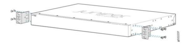
3. Lift the EX3400 switch and position it in the rack. Line up the bottom hole in each mounting bracket with a hole in each rack rail, making sure the EX3400 switch is level.
