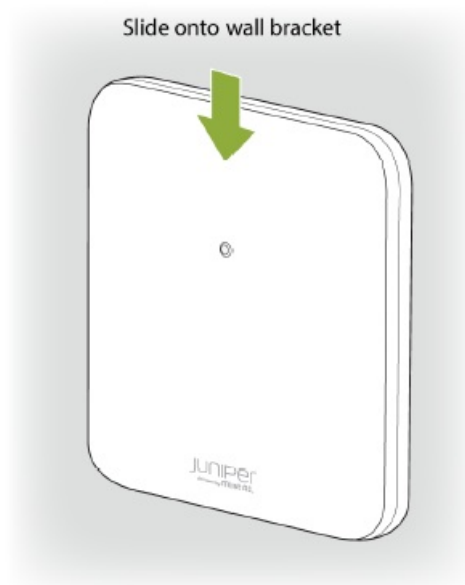
Figure 5: Mount the AP on the Single-Gang Junction Box
