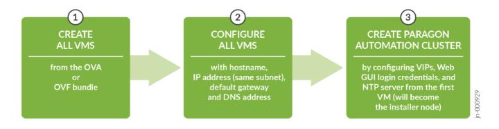
You use the OVA (or OVF and VMDK files) bundle to create your node VMs. The software download files come prepackaged with the OS and all packages required to create the VMs and deploy your Paragon Automation cluster. The VMs have a Linux-based OS of Ubuntu 22.04.4 LTS (Jammy Jellyfish). Once the VMs are created, you must configure each VM in the same way. When all the VMs are configured, you can deploy the Paragon Automation cluster from the first VM.
