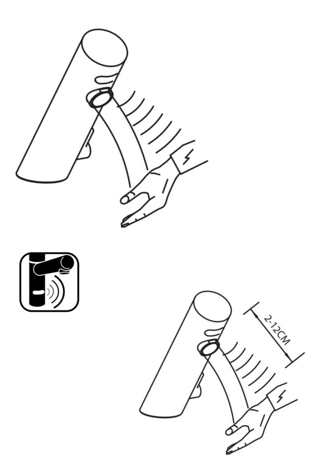
• Hand in detection field of the sensor (2-12cm) -Water starts flowing
