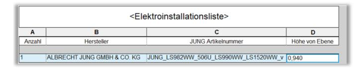
**Attention**: The Elevation from level parameter does not represent the installation height in accordance with DIN 18015-3. To calculate the actual installation height, the combinations contain the installation height distance parameter. This must be added to the Height from level parameter to obtain the actual installation height.
